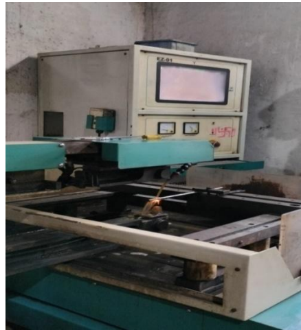
Fig 1 Wire Electric Discharge Machining Experimental Setup
