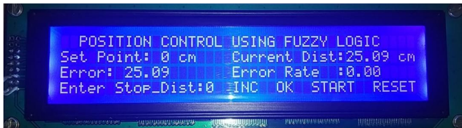
Fig 5: LCD 40 x 4 Character Display
