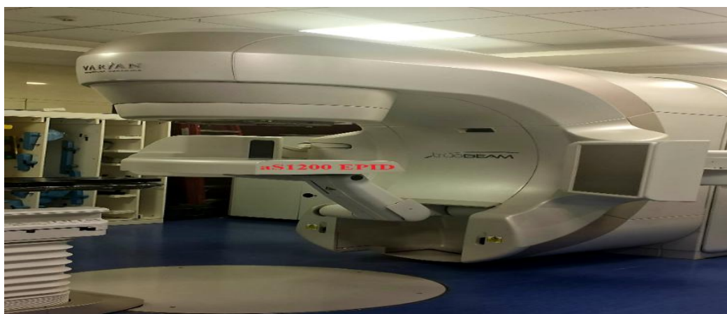
Figure 15 EPID in the planned position to carry out PSQA
