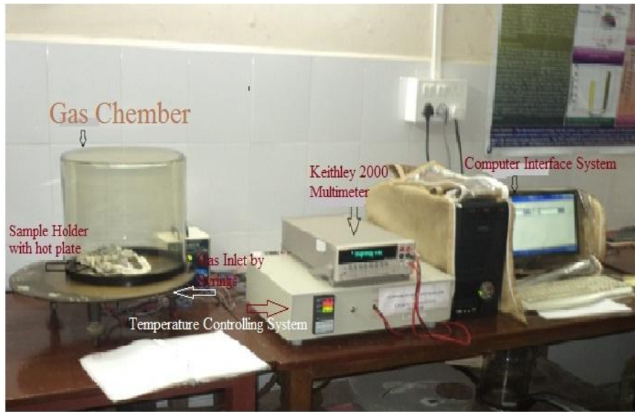
Fig. 4 Gas sensing setup used in present work
